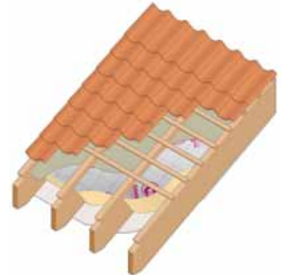
Celotex XR3000 between rafters
