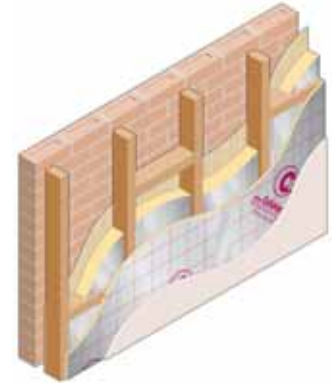
Celotex TB3000 as an internal vapour control layer, preventing thermal bridging
