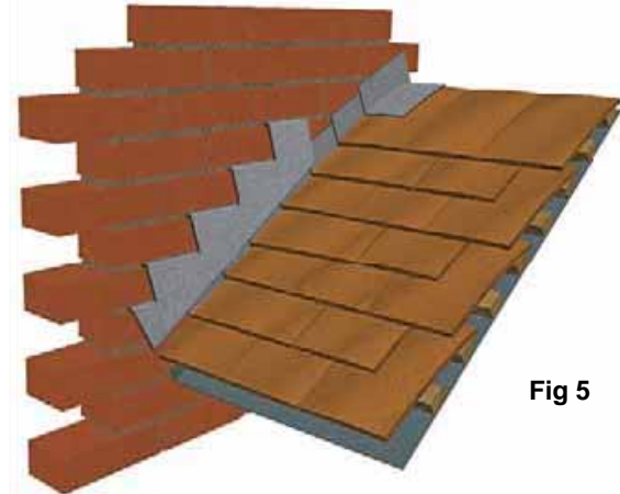
Fig 5: Flashing to a side abutment - double lap tiles/slates
